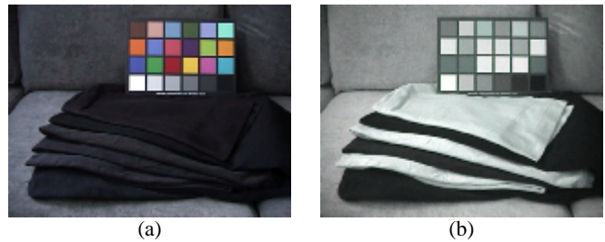
Figure 5: Infrared Reflection of Cloth (a) Six black cloth samples illuminated by daylight, seen in the visible spectrum. (b) The reflection of the same cloth materials under daylight in the near infrared part of the spectrum. The top sample is the one used for the cloth backing in the light stage, just under it is a sample of Duvateen, and the bottom four are various black T-shirts.
