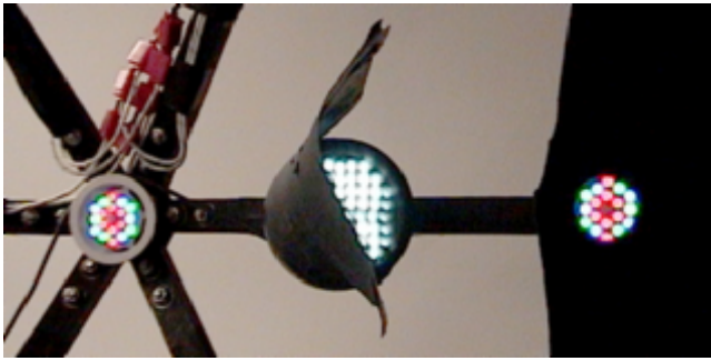
Figure 2: Color and Infrared Lights A detail of Light Stage 3 showing two of the 156 RGB LED lights and one of the six infrared LED light sources. At right is the edge of the infrared-reflective backing for the stage, attached to the fronts of the lights with holes to let the lights shine through. The infrared lights, flagged with black tape to illuminate just the backing, produce light invisible to both the human eye and the color camera used in our system. They do, however, produce a response in the digital camera used to take this picture.
